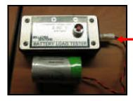
Connect the battery to load tester.
