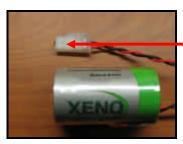
Connect the de-passivation tool to the battery for 5-6 seconds, do not exceed this time or you may reduce the overall battery life.
